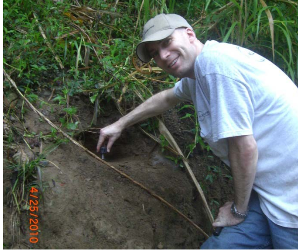
Figure 11-10: Torvane Testing at the Rio Bananito Railway Bridge
