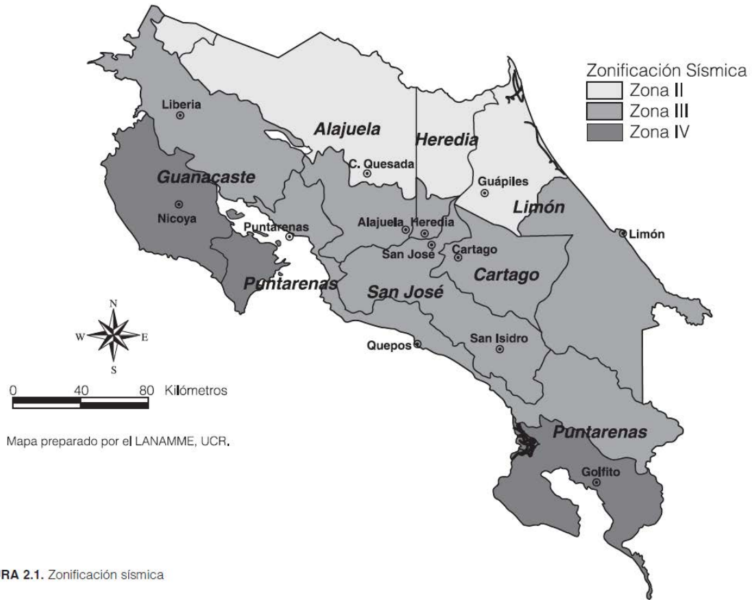
Figure 7: Seismic zoning proposed for Costa Rica (Source: Costa Rican Seismic Code 2002)
