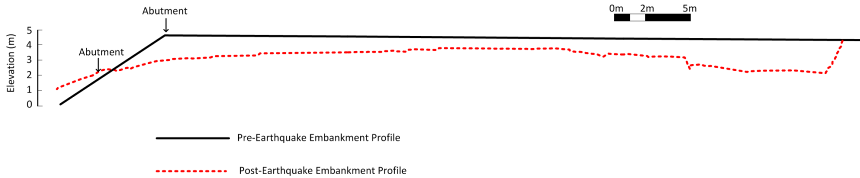
Figure 10-5: Pre- and Post-Earthquake Profile Geometries of the Southern Approach Embankment at the Rio Bananito Highway Bridge
